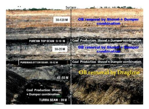
(This diagram, as shown by the appellant during the hearing, shows different coal seams and intervening layers of overburden which are required to be removed before reaching the next level of coal seam. In between Purewa top seam and Purewa bottom seam, shown on the left, there are layers of overburden which is required to be removed before the coal extraction can be done from the next coal seam level)
